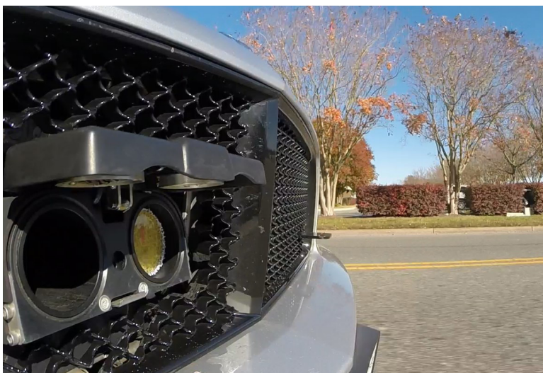
When activated to launch a projectile, the launch door opens. Each unit contains two projectiles to increase the odds to a successful deployment.
